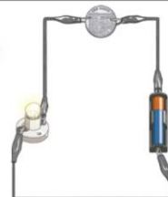
10p = metal = electrical conductors
